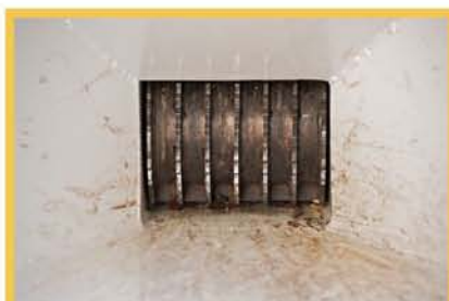
6" x 10" chipper opening to accept forked branches
